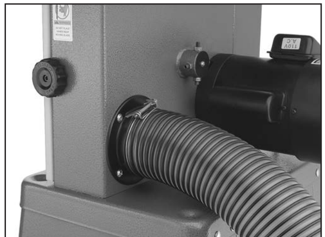
Figure 22. Dust hose attached to dust port.
